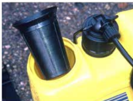
Fig. 8. Engineering controls: enlarged filler opening in a tank and a deep-set filter to avoid splashing of spray liquid
