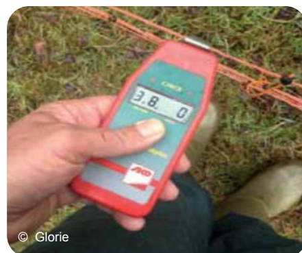
Figure 27. Electric fence - voltage check
