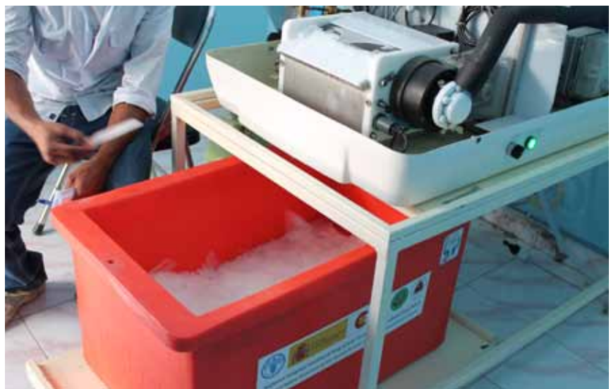
An ice machine installed by RFLP in operation
