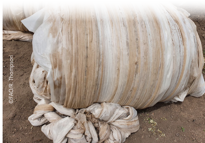
Protective textile removed after one month in the field showing levels of soil contamination, Italy.
