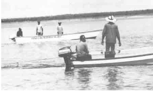
6. (a) MIDWATER PAIR TRAWLING (15 hp units towing midwater trawl. One wooden planked boat built at project. One glass fibre Yamaha 18 ft)
