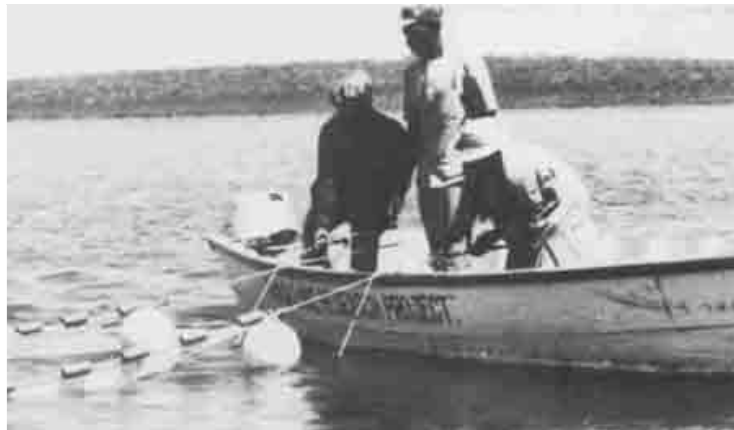
6. (b) MIDWATER PAIR TRAWLING (Hauling the midwater trawl - 15 hp units - the two big floats mark the upper wing tips)
